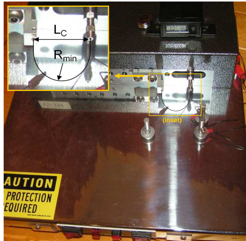
Figure 4.2. Valley Instruments (currently a division of Positool, Inc.) model 10.040 rotating beam fatigue tester.
